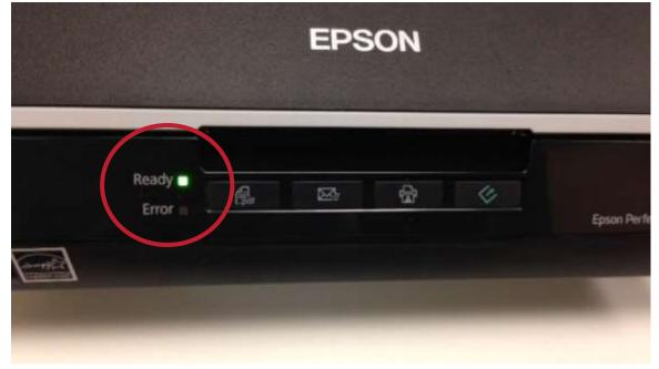
3. If it is not on, press the power button (on the side of the scanner) and wait for the green "Ready" light to stop blinking (when it's a solid light, it's ready to use).
