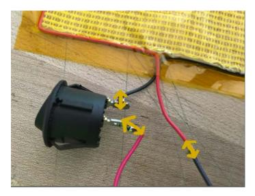
The switch is not polar, meaning it is not positive and negative, so you can choose whichever lead to solder to the battery pack and heating pad.
