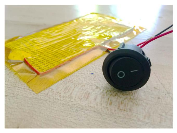
Now you can sew down the heating pad into your clothing. These would be great in the sleeves of a mid-weight winter jacket. Make sure you secure the battery pack and cover the wiring so it doesn't get shorted.
