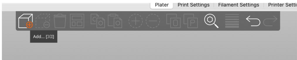
2. **Move/rotate/resize/multiply the print as desired** with the toolbar on the left side of the screen.
